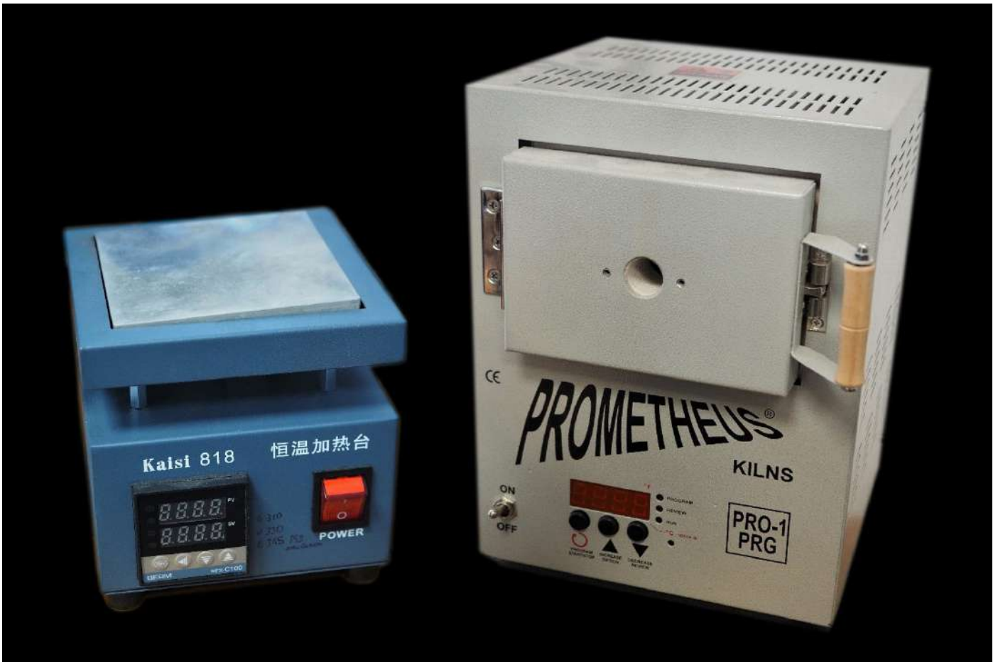
Tools for titanium colouring – a heating plate (left), and an oven
