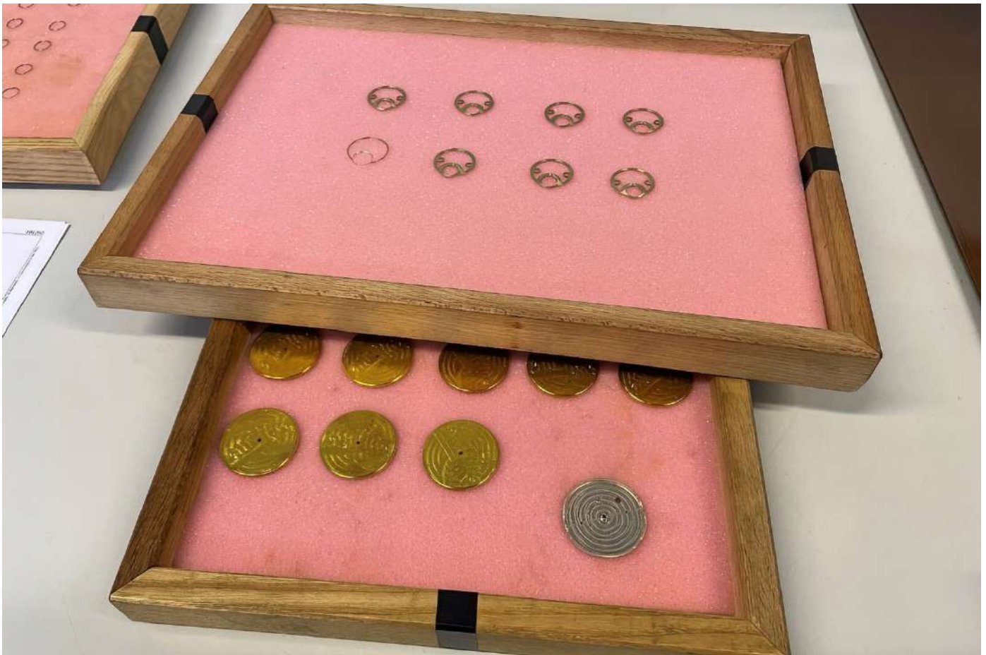
A selection of the many parts constituting the SB05 dial as they emerge from CNC mills (trim ring at top and dial base plate below), with one sample on each tray showing the final stage after finishing has been applied
