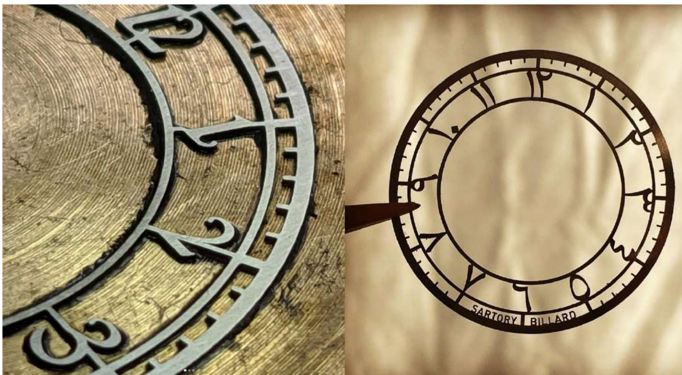
The high level of detail that is possible in the laser-cut chapter ring
