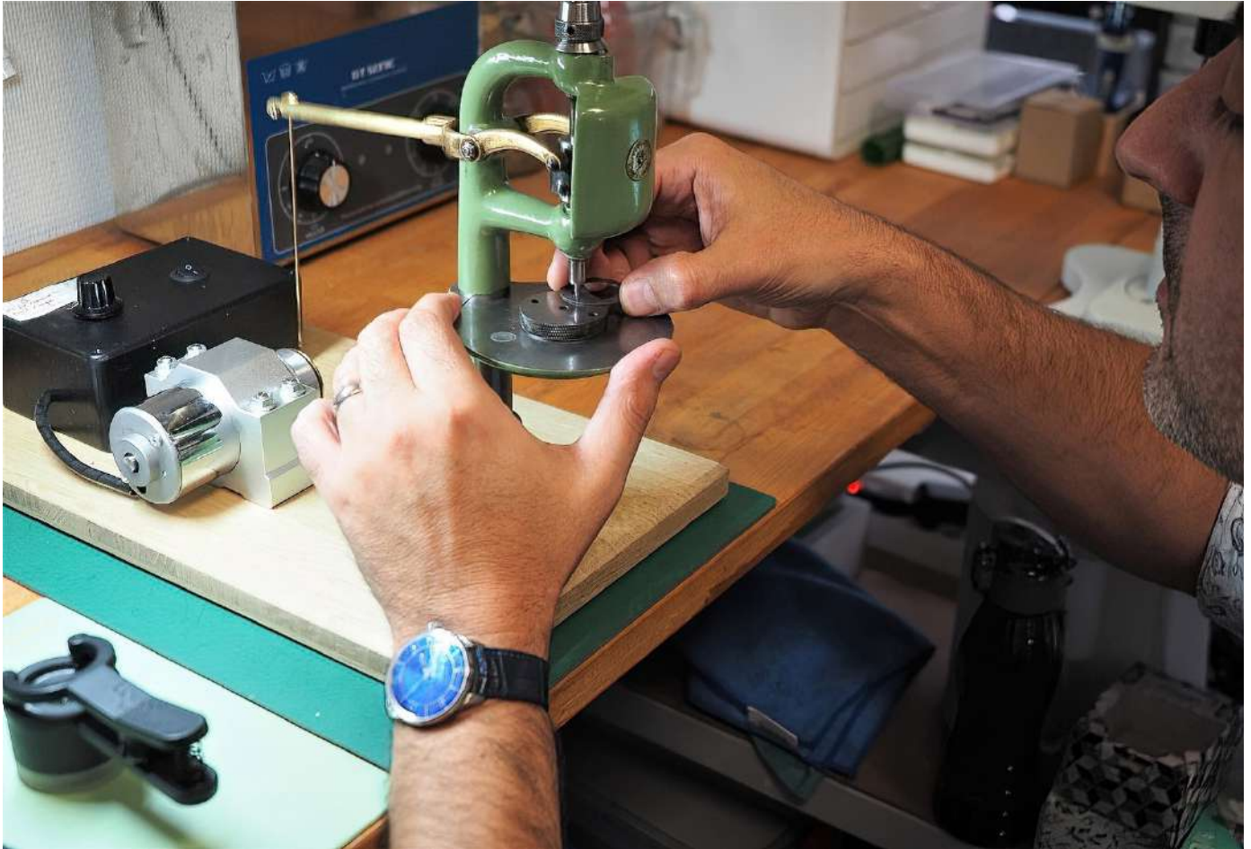
Applying dimples to the dial by hand
