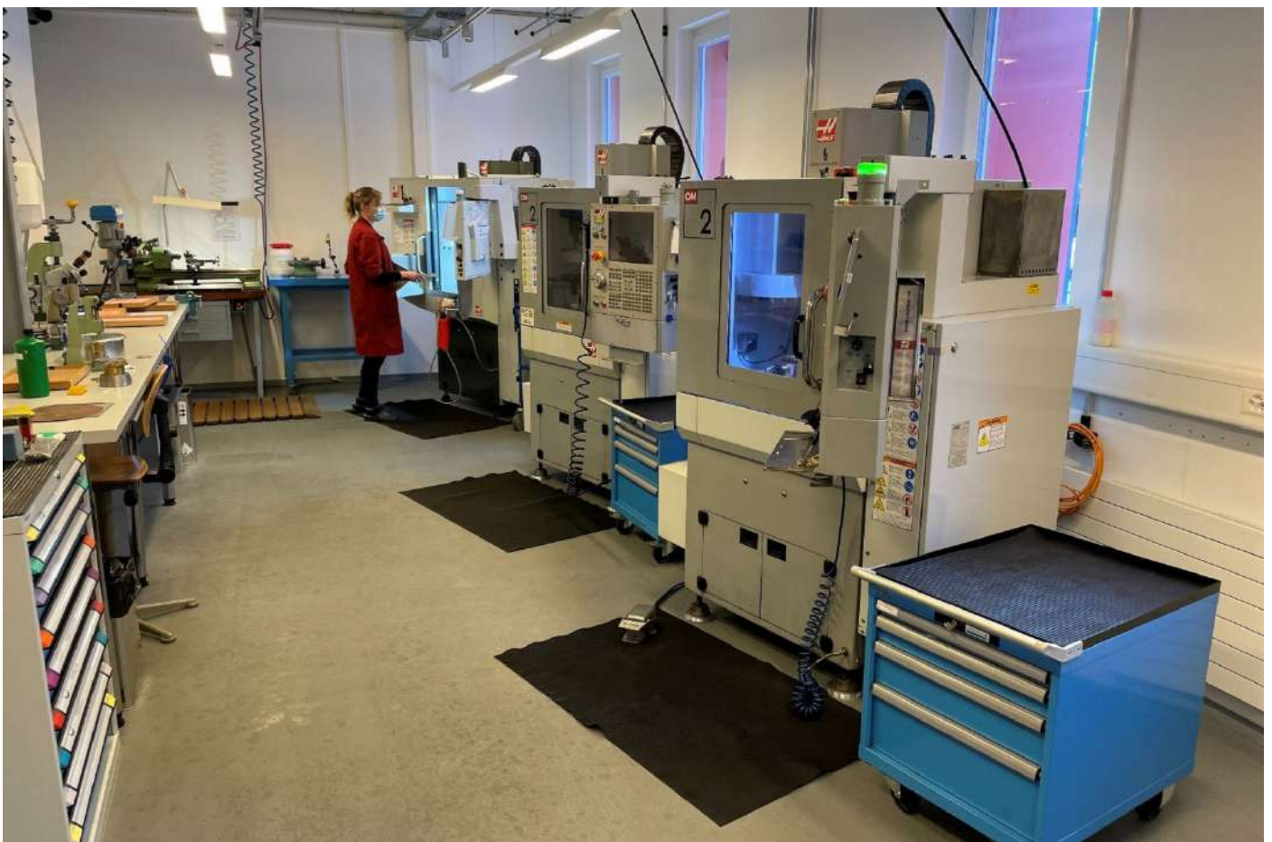
The CNC machines at Comblemine dedicated to manufacturing dial parts. Movement parts, like the basic components for Voutilainen watches, are milled in a separate department.
